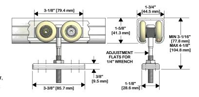
DETERMINE DOOR SIZE/HEADER HEIGHT BASED ON DIMENSIONS SHOWN IN DETAIL VIEWS AND CLEARANCE REQUIRED BELOW DOOR.
